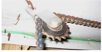
Common vent system problems are loose aircraft cables, rusted vent hinges, worn cable pulleys, rusted chain and sprockets, poorly maintained vent machines and restricted vent inlets. A can of oil and a grease gun go a long way toward extending the life of a vent system. Thumb latches should be installed on every vent door to enable the grower to shut off unused vents when they are not in use.
